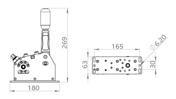
Mount the Q1 Sequential Shifter with 2xM6 or 4xM6 screws.
