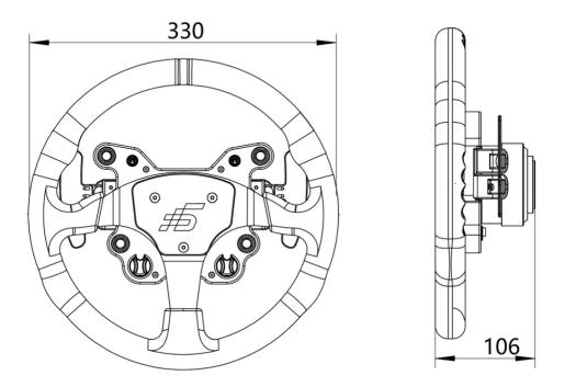
GT1 wheel diameter 330mm Plate mounting hole diameter 70mm PCD; 6xM5\*40 screws Quick Release mounting holes 70x6
