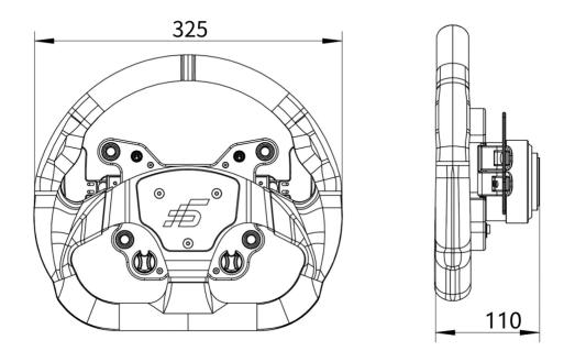
GT1D wheel diameter 325mm Plate mounting hole diameter 70mm PCD; 6xM5\*40 screws Quick Release mounting holes 70x6
